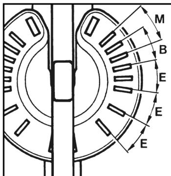
B ➔ Concrete / M ➔ Mortar / E ➔ Emptying
